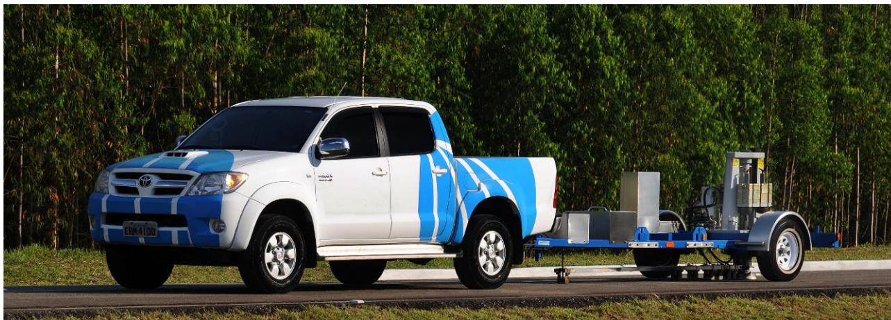
Figura 2 – Vista do Falling Weight Deflectometer Dynatest 8000.
